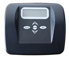
Operating Pressure: 40 - 80 psi Water Temperature: 40 - 80°F Max Inlet Pipe Size: 1"
